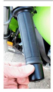
**Step 1**. Grasp bar end to prevent it from rotating. Use a Philips screwdriver to remove the bar end.
