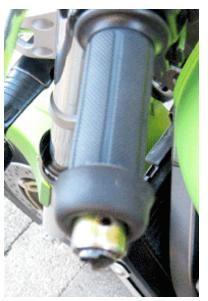
**Step 2.** On the clutch side, roll back end of grip to expose the holes in handlebar. On the throttle side, remove the throttle tube assembly to expose holes.
