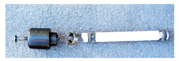
This photo shows the components that will be removed. From left to right: Philips screw – bar end – internal weight retaining clip – internal weight assembly
