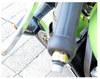
**Step 3.** The internal weight assembly can now be slid out of the bar. You can use the Philips screw that held on the bar end as a handle if the weight assembly does not slide out easily. If you have lost the screw or do not want to risk damaging it with your pliers or vice grips, it is a 6mm screw.
